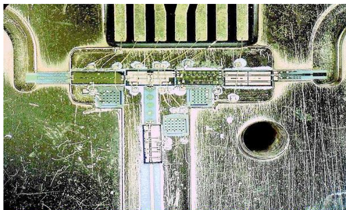
Figure 4. 100-140 GHz Module Picture of Downconverting Block
