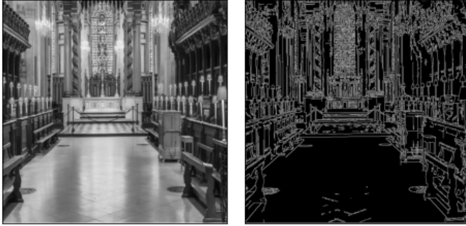
FIGURE 1. Left side, the original image. Right side, edges obtained by using a Canny edge detector.
