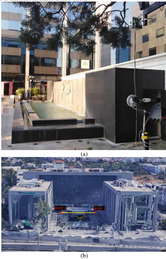
Fig. 5. Outdoor measurements setup across the water to see the direct path and the reflected path, distance between the nodes is 24m (a) Node-I mounted on a pole at a height of 3m (b) Node-II is placed outside the building and mounted on a tripod at a height of 3m.
