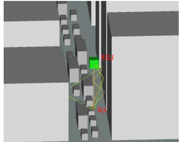
FIGURE 3. Illustration of the deployment of ray tracing simulation. Small cars and trucks are randomly dropped in the two lanes of the urban canyon. Receivers are mounted on the top center of the small cars, and the BS is denoted by the green box. The figure displays the five strongest paths of the channel for a NLOS receiver. It is shown that multiple reflections happen on the buildings and the vehicles.
