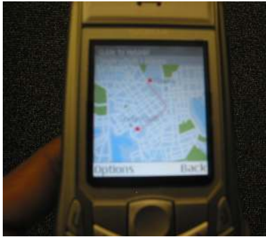
Figure 7: Camera-based interaction in a map viewing application. The map is rendered using vector graphics, so it can be scaled with no loss in quality. Physically-based scrolling and zooming coupled with vector graphics creates a better navigation experience for users.
