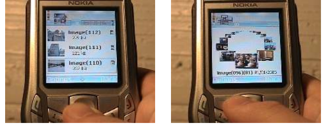
Figure 1: Picture browsing task. Left: traditional list view, Right: 3D image carousel. Browsing a large collection of images is difficult using conventional approaches as the user's attention is focused on controlling views instead of their objectives.
