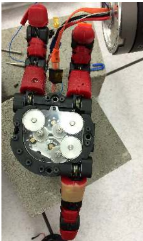
(a) RoboSimian hand with drive gears exposed. Note the staggered opposing fingers.
