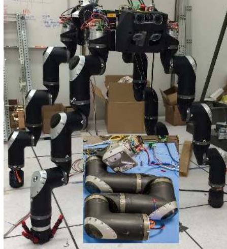
Figure 3: RoboSimian's limbs extended with inset showing a compact folded limb.
