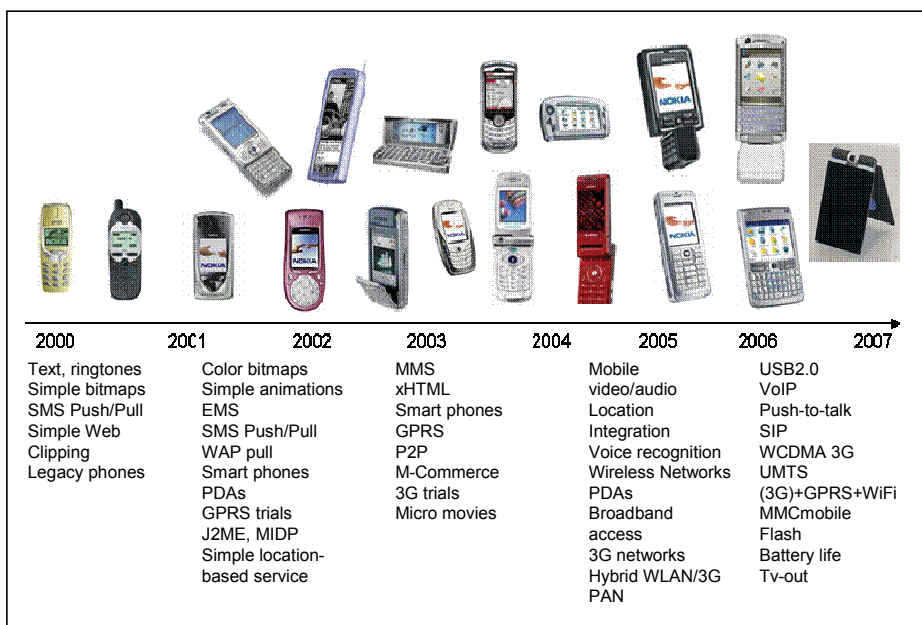
Fig. 4. Development of mobile handsets (modified from Karjaluoto et al. 2006).
