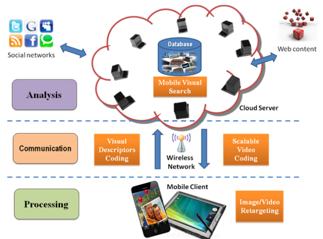
Figure 1. Mobile Media Communication, Processing, and Analysis visual search and augmented reality applications, such as CD/Book cover search, location recognition, scene retrieval, product search, etc.
