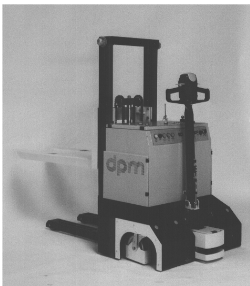
Figure 5: Typical industrial Autonomously Guided Vehicle (AGV) used for demonstrations of a forklift handling device and optical line following system.
