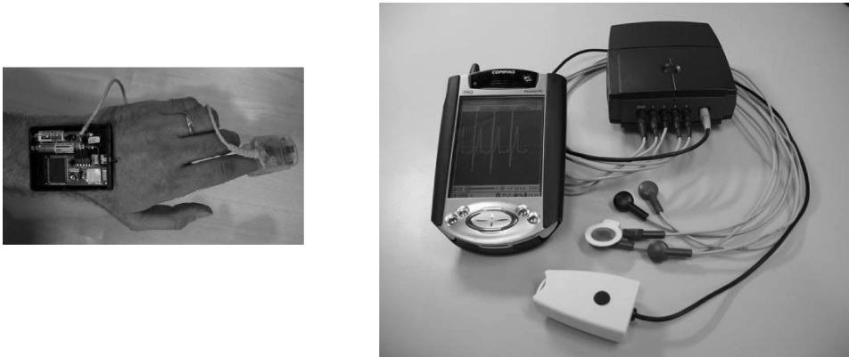
Figure 3. Self supporting sensor (left) and complete front-end system with ECG and oxygen saturation sensors
