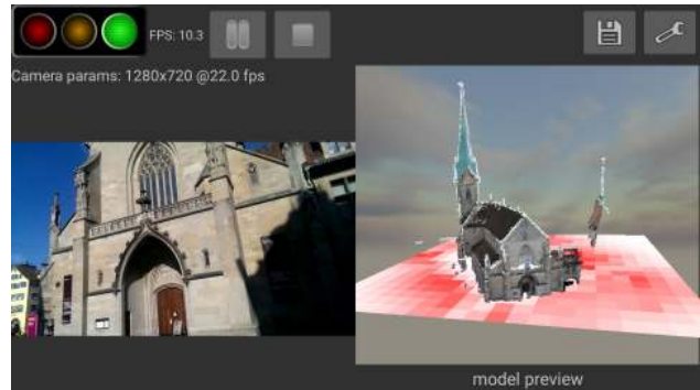
Figure 1: Screenshot of Android mobile frontend: Live camera preview (left) and current 3D reconstruction and next best view guidance (right). A traffic light symbol indicates the status of the tracker and reconstruction quality.
