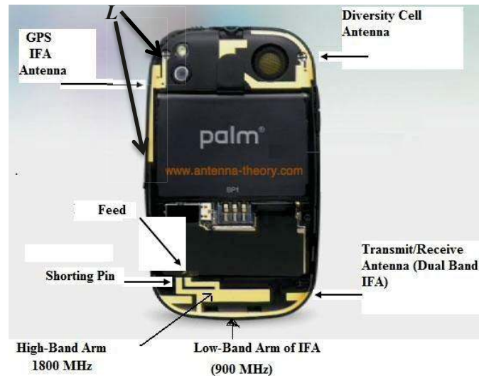
Figure 3.1.1 Palm Pre Antennas viewable by Removing Back Cover.
