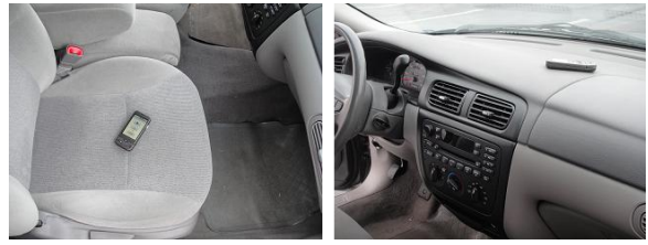
Fig. 5. The G1 phone is put on the front seat or the dashboard of the vehicle during drunk driving detection.
