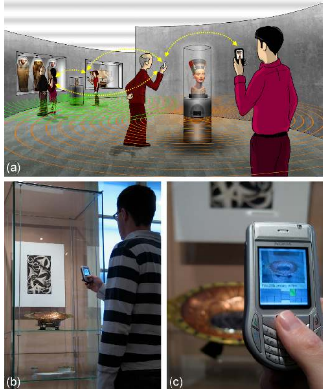
Fig. 1. Basic concept (a) and application (b,c) of the PhoneGuide system in a museum: Adaptive classification in dynamic large-scale museum environments supported by ad-hoc sensor networks and phone-to-phone communication.
