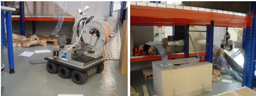
Fig. 1. A rescue robot with the glassfibre drum on its back (left). It has to operate in an environment where high mobility is needed and the glassfibres are experiencing a lot of stress through obstacles (right). Nevertheless, the glassfibres never failed in over two years of operation.
