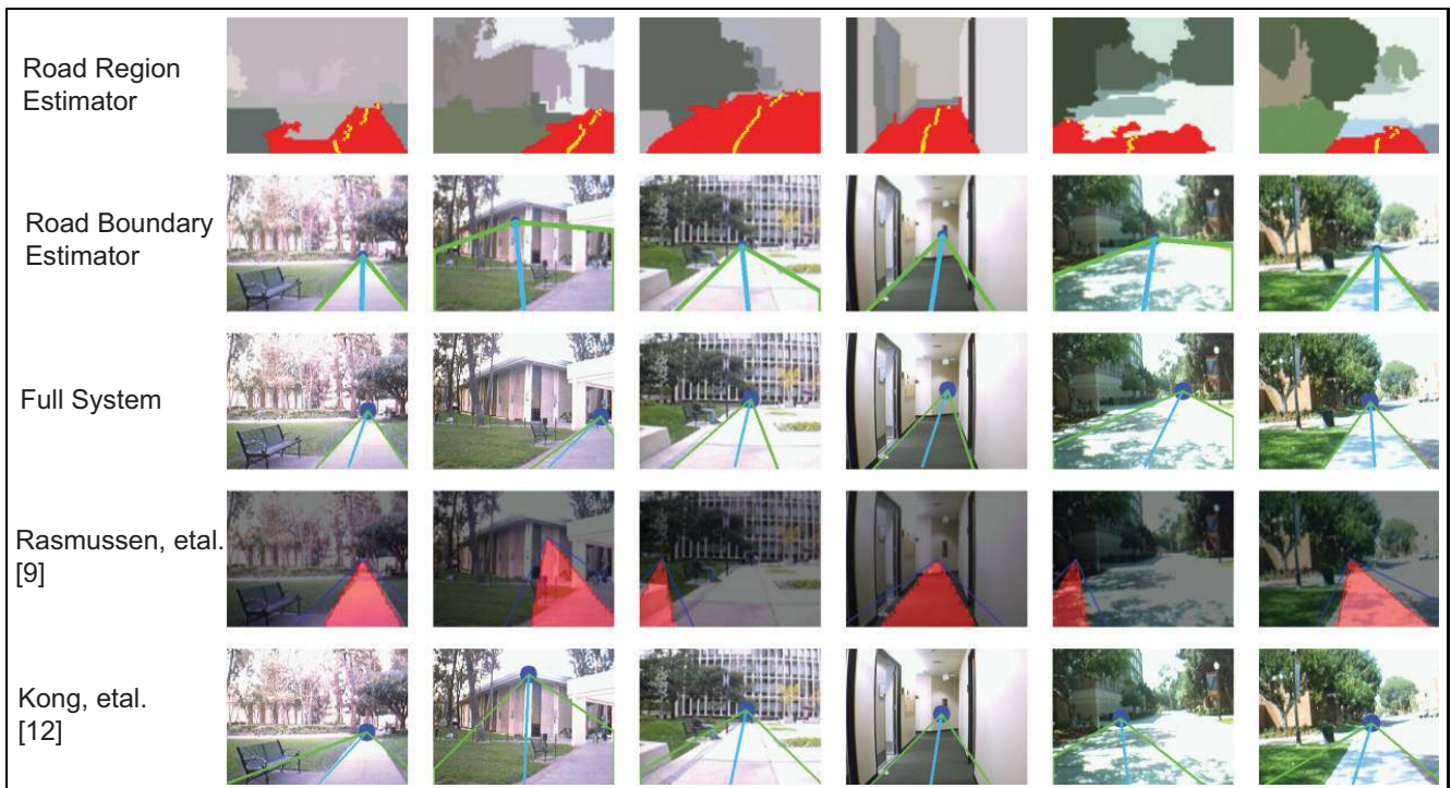
Fig. 9. System Comparison Examples. The different systems outputs are organized to different rows with the first three rows occupied, in order, by the individual algorithms in our approach, road color region detection and road boundary estimation, and then the overall system. In addition, we also include an implementation of systems by [9] (forth row) as well as [12] (fifth row).
