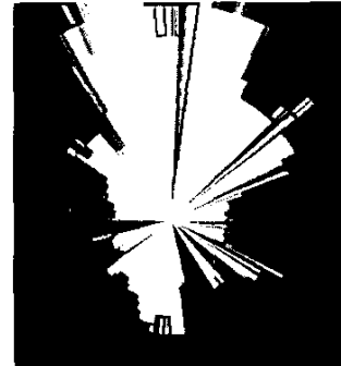
Figure 6: An example map. The white region indicates the free space; gray regions indicate the areas where observation counts are less than the threshold; black regions indicate the area where the observation is never counted.
