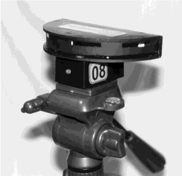
Figure 8. Stationary NOADs are located at known positions; at least two NOADs are networked and connected to a PC (courtesy of MTI Research Inc. 19a ).
