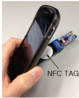
Figure 2. Initiating connection process
