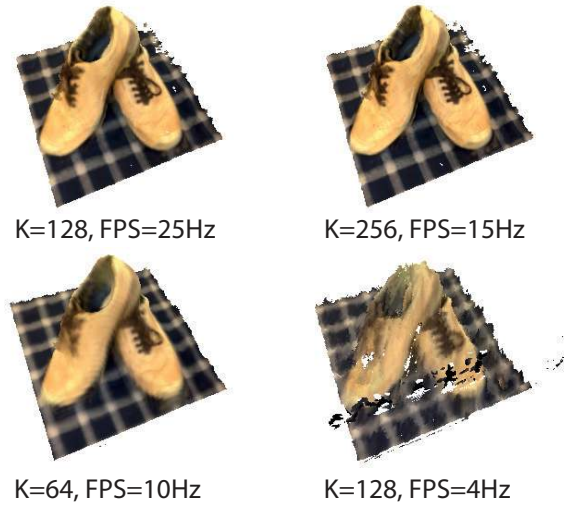
Fig. 7. Effect of different model resolution and FPS on model quality. Our current implementation supports K = 128 at 25Hz and K = 256 at 15Hz. Note that processing speed is however the more dominant contributor to model quality. This is because at higher frame-rates, the redundancy of depth maps fused volumetrically leads to greater denoised results even at lower resolutions.
