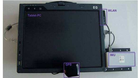
Fig. 5. Tablet-PC with the u-blox-GPS receiver, the WLAN-Card, and the IMU iSens-3.
