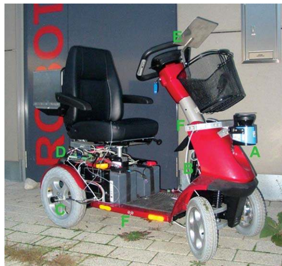
Fig. 1. The mobility scooter equipped with all electronics and sensors A) Laser Range Finder, B) steering motor, C) incremental sensor, D) electronics, E) mounting device of the navigation system, F) ultrasonic sensors.
