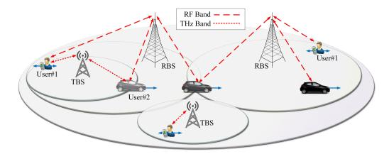
Figure 1. Graphical illustration of a two-tier hybrid RF-THz network with low- and high-velocity users.
