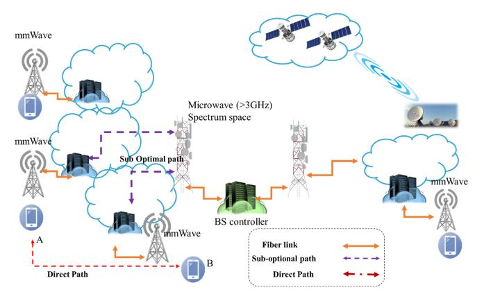
Figure 6. A distributed network that places content servers in the access network.
