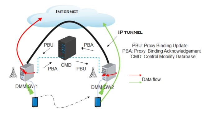
Figure 7. PMIPv6-based DMM.
