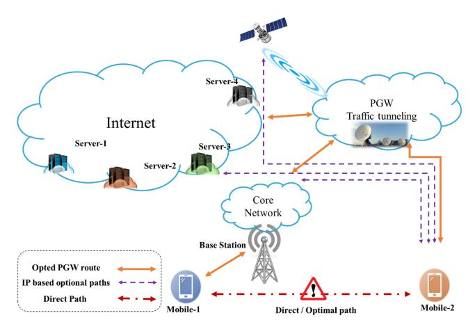
Figure 1. Centralized mobility IP data flow management.
