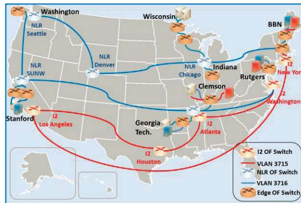
Fig. 17: Physical network configuration during GENI proof of-concept demonstration
