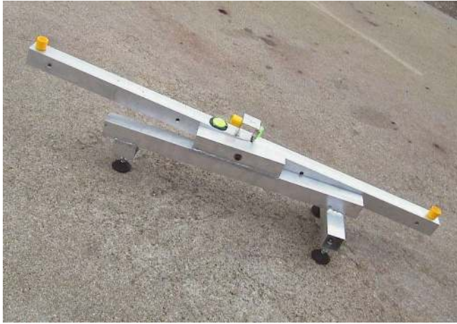
Figure 4. Support structure for response measurements.
