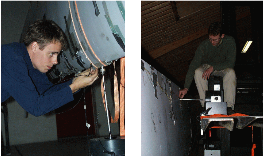
Figure 26. Vertical and horizontal forcing applying an electromagnetic exciter.
