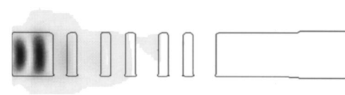
Fig. 8. Semiconductor waveguide core with air on both sides and the photonic crystal holes etched right through the core. The magnitude of the magnetic field, enhanced to show cavity losses, is plotted for one side of the symmetrical cavity.
