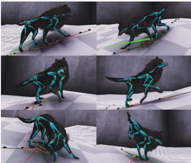
Fig. 7. The quadruped character walking over a smooth uneven terrain synthesized by full-body inverse kinematics.
