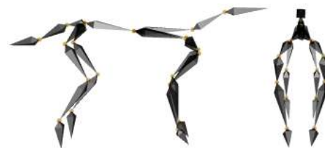
Fig. 4. The skeleton structure of the dog model used in our experiments. It is composed of 27 bones and has 81 degrees of freedom in total.
