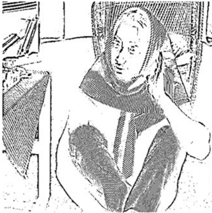
(a) Edge-detection is preserved in the residual which is obtained by subtracting all the functional modes from the original image. The functional modes are separated using the single MoDEE algorithm with repeated application and different diffusion constants and evolution time. Lines are fine and continuous characterized as good edge detection.
