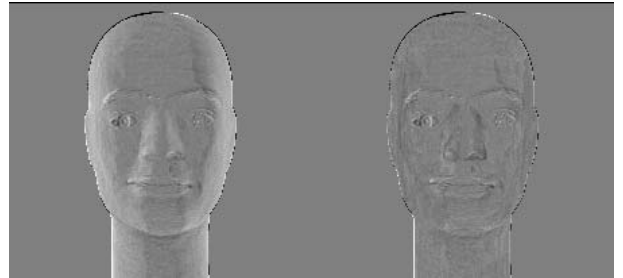
Figure 5: Frame difference after motion and global illumination compensation (left) and frame difference with Lambertian approach for illumination compensation (right).
