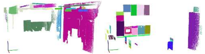
Fig. 12. Vertical planar regions classified as: walls (left); furniture candidates (right); for the dataset presented in Figure 1.
