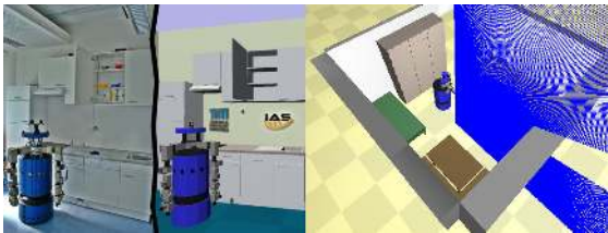
Fig. 11. An illustration of the simulated 3D environments and the process of acquiring training datasets, using the Gazebo 3D simulator.
