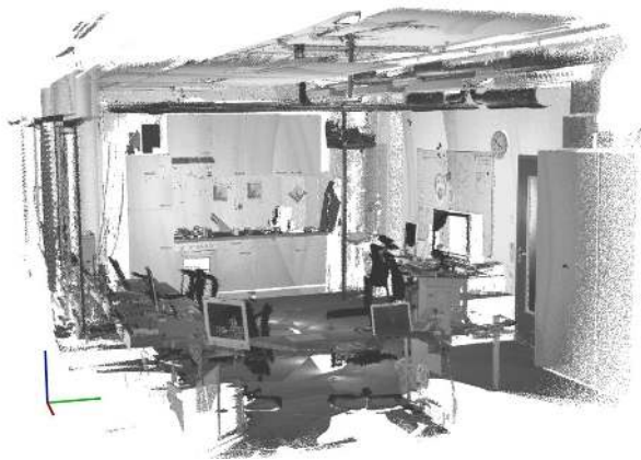
Fig. 1. A snapshot of our kitchen lab: 16 registered scans shown in intensity (grayscale), comprising roughly 15 millions of points. The world coordinate system depicted on the bottom left shows X with the red color, Y with green, and Z with blue.
