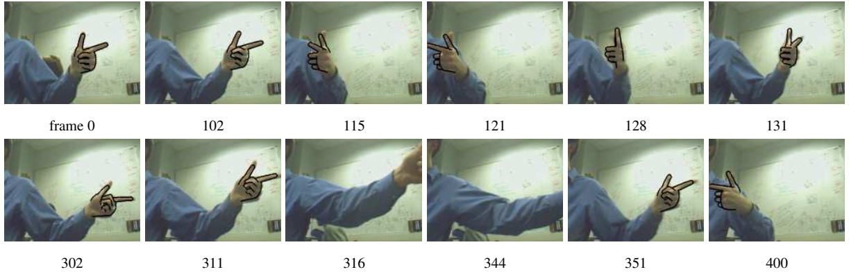
Figure 8: Fast motion and recovery. This figure shows frames from a sequence tracking 6 DOF. (Top row) The hand is tracked during fast motion and (bottom row) the tracker is able to successfully recover after the hand has left the camera view.
