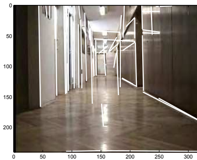
Fig. 18. Superposition of camera view and line segments extracted by RWRHT method
