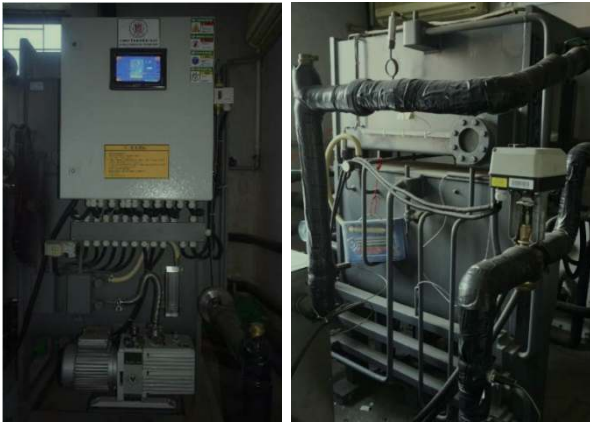
Fig.6 Picture of the single effect absorption chiller experimental platform (left: front, right: back)
