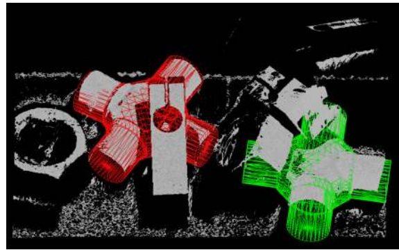
Figure 1. Example of two partly occluded instances of an object found in a noisy, cluttered scene. The matched objects are shown as red and green wireframe and might not be recognizable in B/W copies.
