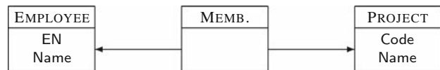
Fig. 2 The translation of the schema in Fig. 1 into a simple object-oriented model
