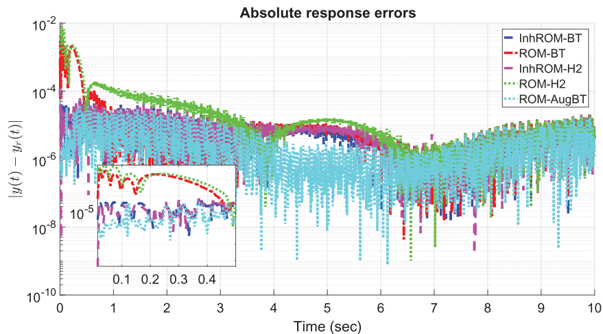
Figure 3. Absolute response errors of the reduced-order models of the nonlinear RC circuit with a fixed initial condition ( \alpha = 1 ).
