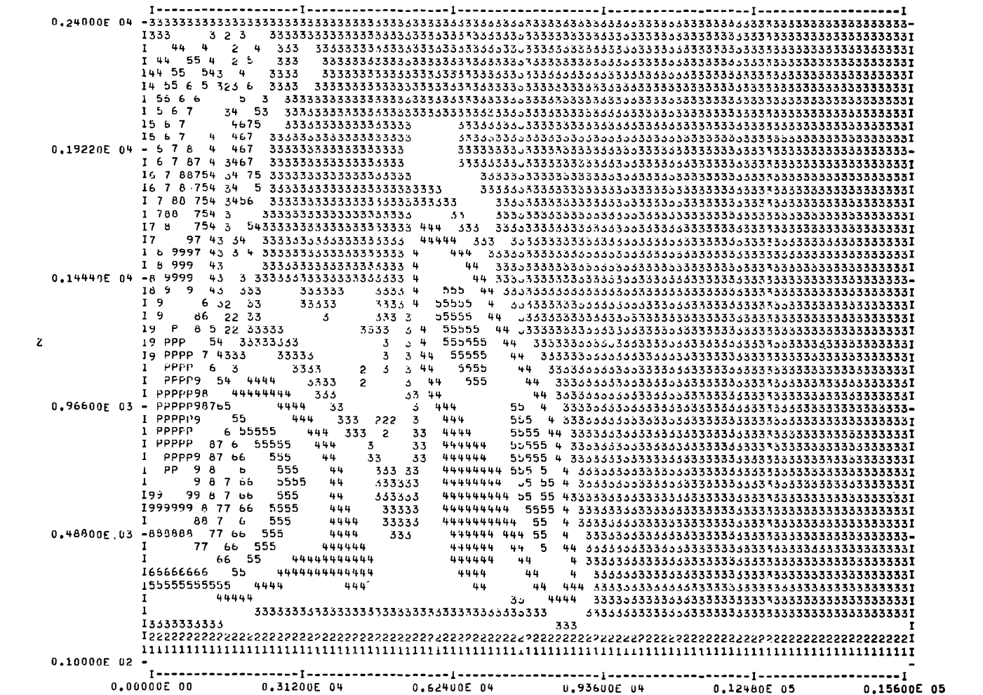
Figure 4.4.7. Normalized scale of turbulence contours as a function of z and y for a two-dimensional gust front with a 2000 m radius downdraft at t = 1000 sec. [See figure 2.3.2 for explanation of notation.]
