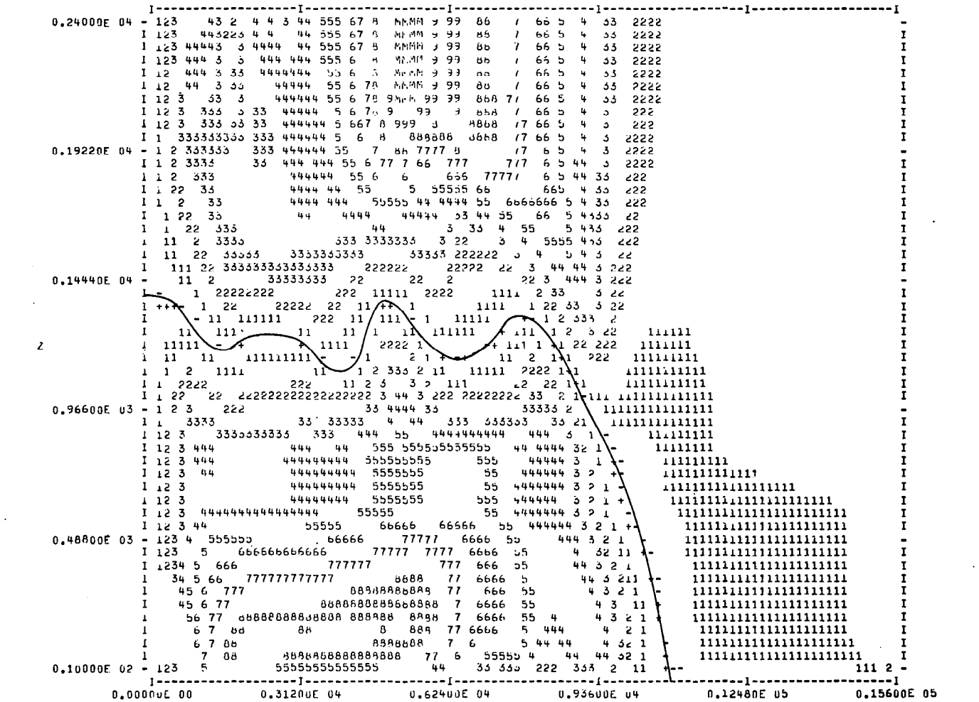
Figure 4.4.4. Normalized mean radial velocity contours as a function of z and y for a two-dimensional gust front with a 2000 m radius downdraft at t = 1000 sec. [See figure 2.3.2 for explanation of notation.]
