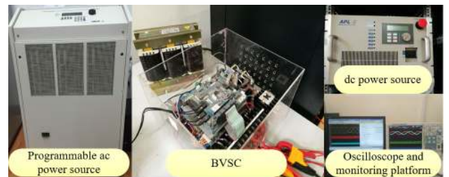
FIGURE 4. Experimental setup of fault-tolerant BVSC.
