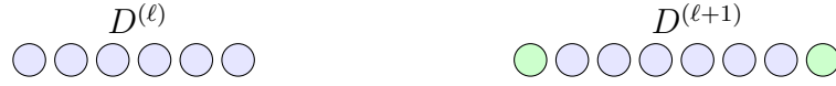
Figure 4.1: \leftarrow Extension of one-dimensional support approximation done by adding two states (green) on the left and on the right.
