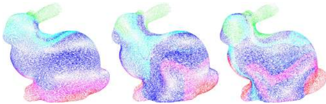
Figure 4: Curved domain: While all other figures were achieved on a regular grid, our approach applies to arbitrary domains, here on the surface of a triangulated domain; a simple laminar flow with initial horizontal velocity smoothly varying along the vertical direction quickly develops vortical structures on this complex surface.
