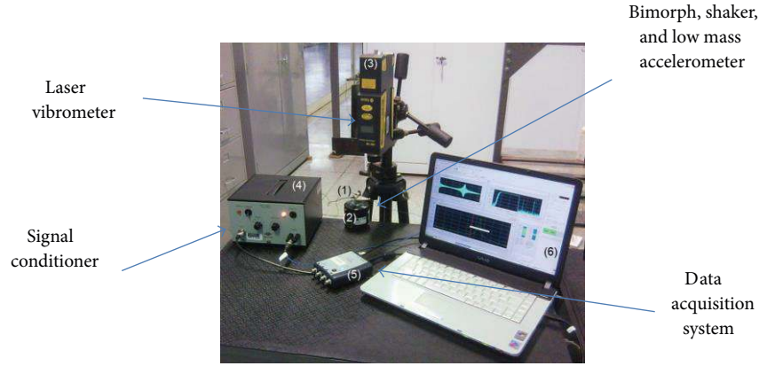
FIGURE 3: Experimental setup used for the verification of relations for a tapered beam.
