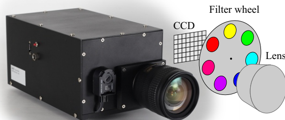
Figure 1: Our multispectral camera, using 7 optical filters. Its internal configuration is sketched.
