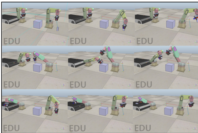
Figure 8: Coordination of Robotic arm in V-REP obtained from importing simulink model.
