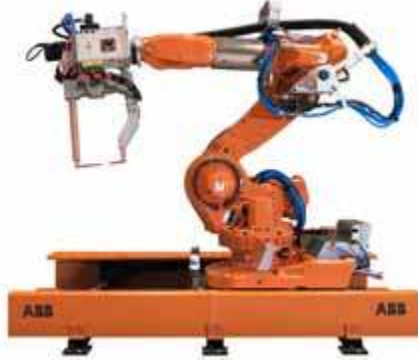
Figure 3.3: A robot moved by a track motion.
