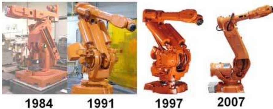
Figure 1.1: The development of large ABB robots. 1984: IRB90 1450 kg and payload 90 kg (16:1), 1991: IRB6000 1750 kg and payload 120 kg (15:1), 1997: IRB6400R 2100 kg and payload 200 kg (10.5:1), 2007: IRB6640 1300 kg and payload 235 kg (5.5:1)
