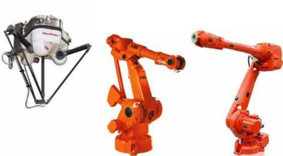
Figure 2.2: Three examples of robot structures from ABB. The parallel arm robot IRB340 (left), the parallel linkage robot IRB4400 (middle), and the elbow robot IRB4600 (right).
