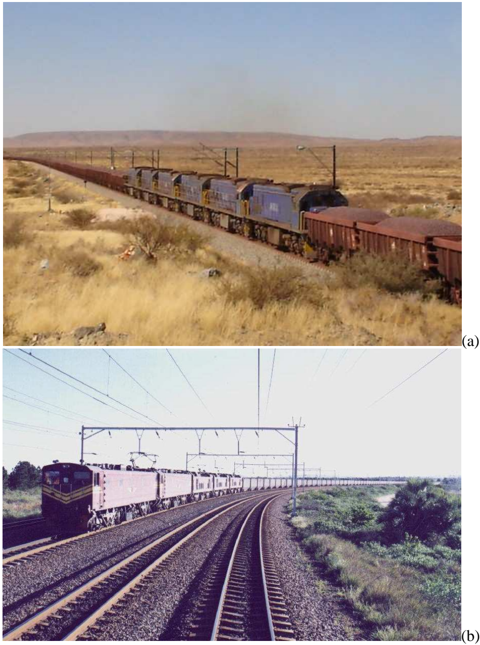
Figure 1. Heavy haul trains of Spoornet, South Africa. (a) is a heavy haul train transporting iron ore, and (b) is a heavy haul train transporting coal in the COALink line of Spoornet. Such a heavy haul train usually has about 200 wagons that stretch 2.5 kilometers. Extremely long trains up to 10 kilometers in length are considered in the business plan of Spoornet.
