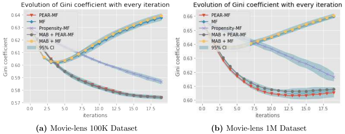
Figure 22. The evolution of the Gini Coefficient is tracked after each iteration. PEAR-MF is decreasing the Gini coefficient after each iteration which proves that it is contributing to decreasing the imbalance in the data
