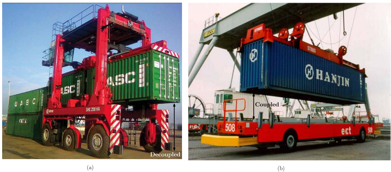
Figure 1 a) Automated Lift Vehicle (ALV) (source: www.sae.org ), b) Automated Guided Vehicle (AGV)
