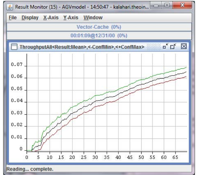
Fig. 4. Result monitor showing the transient evolution of overall throughput with confidence intervals
