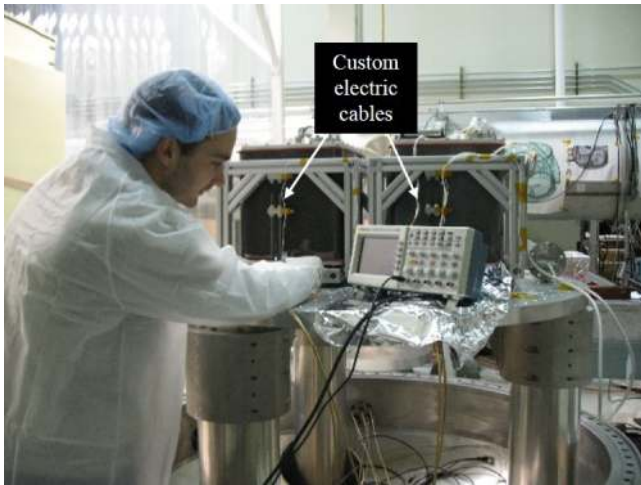
FIG. 20. Custom electric cables routed along the suspension wires.
