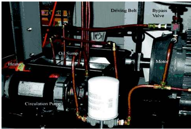
Fig. 8 Photograph of the circulation system. The oil sump is heated if required. The circulation pump maintains the oil temperature while the motor rotates one plate.
